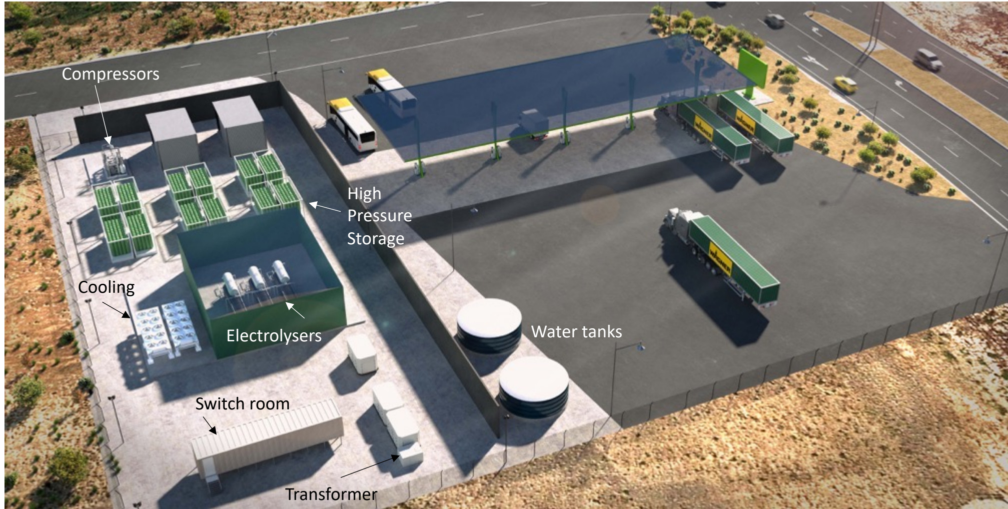
Lion's concept design of a hydrogen production hub with collocated refueling facilities
